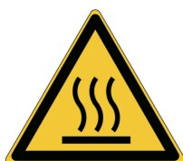
Figure 26: This symbol is used on the pre-humidifiers to warn for high temperatures.
