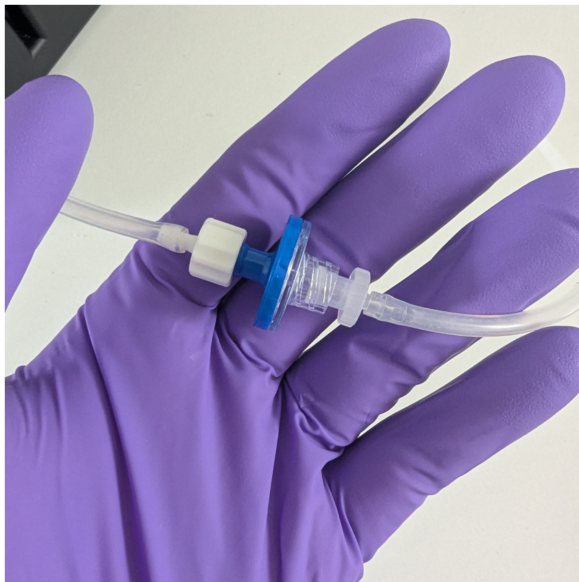
Figure 23: Hydrophobic filters are used to ensure safety of the pumps and sterilise the air input. These should be placed in the line prior to pre-humidifier flasks. Note that they will not prevent backflow, but will prevent liquid ingress into the sparging pumps.
