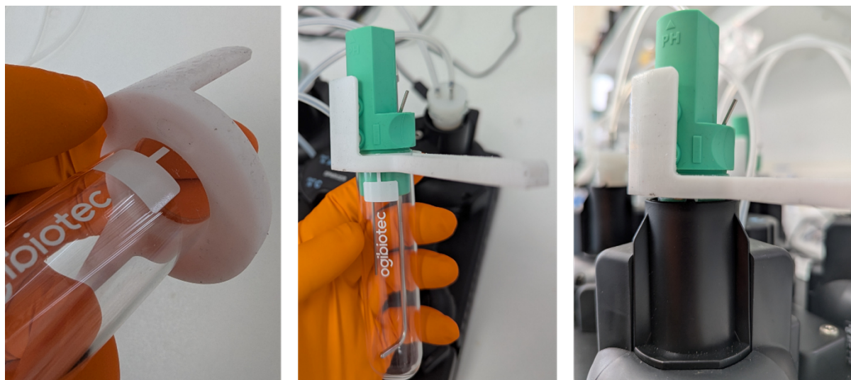
Figure 25: Correct application of the spill guards to the top of the OGI3 culture flask. Note that the inset portion on the underside of the spill guard should line up with the marker on the culture flask. The bung may then be aligned with the same marker for complete alignment of the now guarded culture flask.
