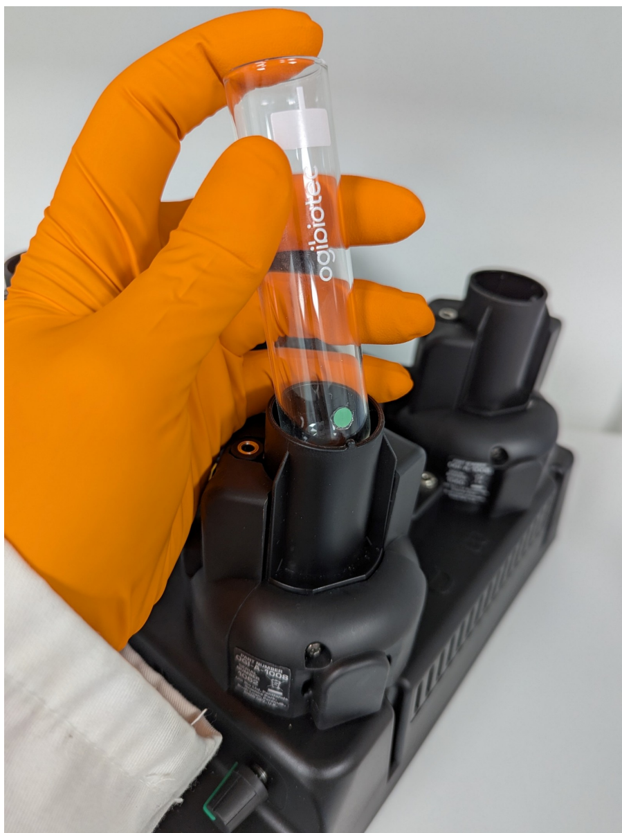
Figure 16: Correct alignment of oxygen sensor spot – Spot to notch in flask holder
